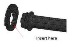
• Connect the two cables of the throttle control to the lower half knob, make sure you insert the forward and backward cables correctly.
